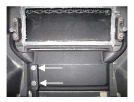
6. Completely remove the rear bolt from each of the bypass retainers, and loosen the front bolt using a 1/2" wrench. It may be necessary to remove the center 1/4"-20 x1" bolts, (loosen lock nuts first) using 7/16" socket or wrench, to access them. Twist the retainers out of the way and remove the bypass cover.
