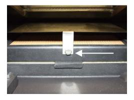
11. Replace the cover plate using 5/32" allen wrench.
