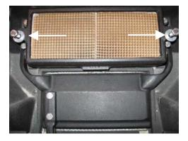
5. Detach the bypass lift guide by removing the two bolts that attach it to the top side of the bypass door using ½" wrench or socket.
