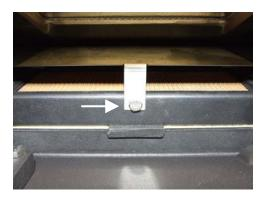
4. Pre-treat all hardware to be removed with a penetrating liquid. Let stand for 15 minutes. Do not spray penetrating liquid directly on the catalytic combustor. If you have not already done so, remove the two transport bolts that hold the combustor assembly in place using ½" wrench or socket. (These bolts do not need to be reinstalled as they are for transport only). Remove the combustor and frame assembly from the stove.
