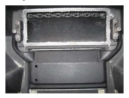
8. When installing the ¼"-20x 1" bolt in the center of each retainer, pull the bypass door upward so that it is pressed against the under side of the retainers. With the door held in this position tighten the middle bolt until it just touches the door hinges. Now you may release the door. Tighten the bolts one full revolution using the bolt code on the bolt head for easy positioning reference. Tighten the lock nut to keep the bolts in that position.
