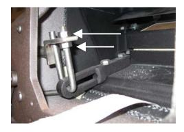
10.Place the combustor assembly back into position and place the heat shield back into position.
