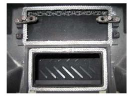
7. Place the new bypass cover into position. Apply anti seize compound to the bolt threads. Swivel the retainers back into position, and secure them with the bolts provided.
